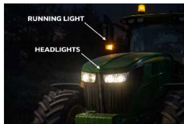
Figure 2.9.3 Close-up of a tractor at night, highlighting its headlights and running light with labels pointing to each.
