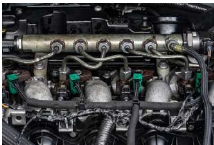
Figure 2.11.1 Close-up of an engine's fuel injectors, featuring metallic components and green connectors, with wiring and hoses visible.
