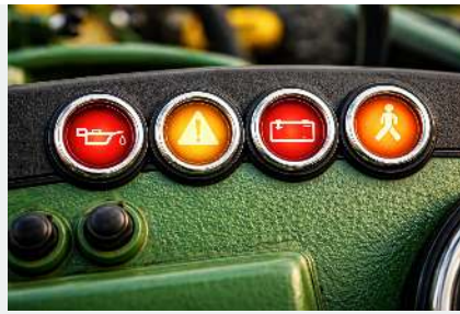
Figure 1.9.4 Control panel with four warning lights: oil level, general alert, battery status, and a pedestrian symbol.
