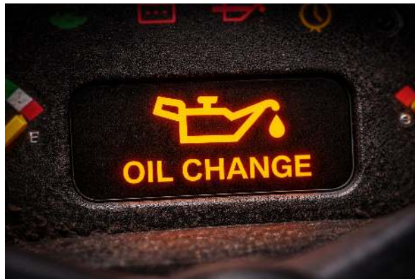
Figure 7.7.1 Illuminated dashboard warning indicating an oil change is needed, featuring an oil can icon and the text "OIL CHANGE."
