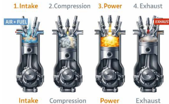
Figure 2.3.1 Illustration of a four-stroke engine cycle: Intake, Compression, Power, and Exhaust phases labeled accordingly.
