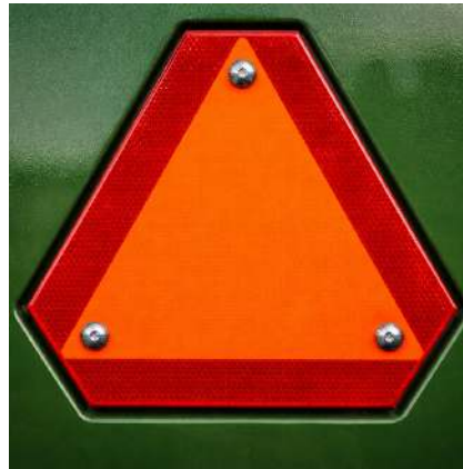
Figure 6.3.3 Reflective orange triangle warning sign bordered by red, mounted on a green surface.
