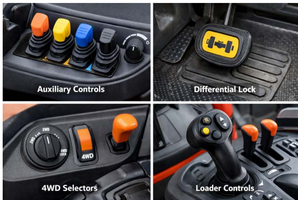
Figure 4.16.2 auxiliary controls, differential lock, four-wheel drive selector, and loader controls
