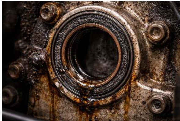
Figure 8.1.1 Close-up of a metal engine component with an oil seal, showing dirt and oil residue around it.
