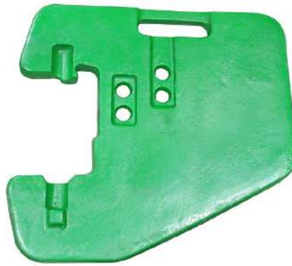
Figure 3.14.1 Green metal ballast made to attach to the front end of a tractor to add extra weight to the front wheels to assist in better steering traction.
