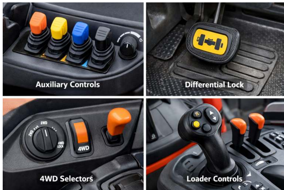
Figure 4.9.1 auxilliary controls, differential lock, four-wheel drive selector, and loader controls
