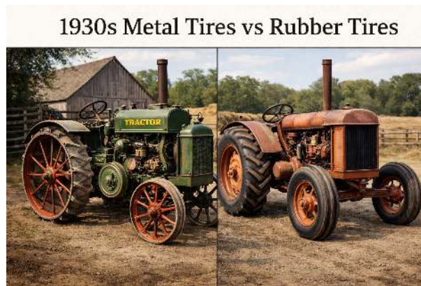
Figure 1.2.4 Side by Side Comparison of tractors with metal tires and rubber tires.
