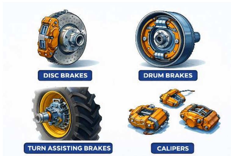
Figure 3.12.2 Illustration of various brake systems: disc brakes, drum brakes, turn assisting brakes, and calipers with labels.
