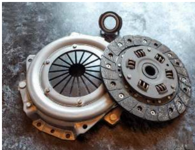
Figure 3.2.2 Close-up of a car clutch assembly, showing the pressure plate and clutch disc on a textured surface.
