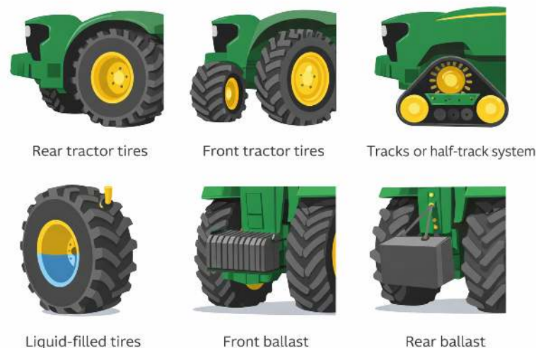
Figure 5.10.1 Illustration showing different tractor components: rear and front tires, tracks, liquid-filled tires, and ballast systems.
