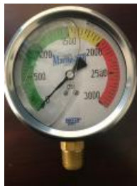
Figure 4.7.1 A pressure gauge with a dial showing green, yellow, and red zones, indicating pressure levels from 0 to 3000 psi.
