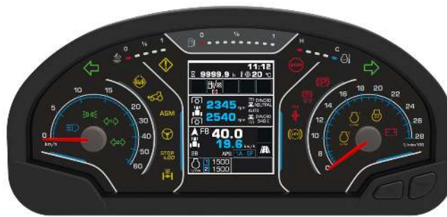
Figure 4.8.1 Dashboard display with speedometer, fuel gauge, and various warning indicators.
