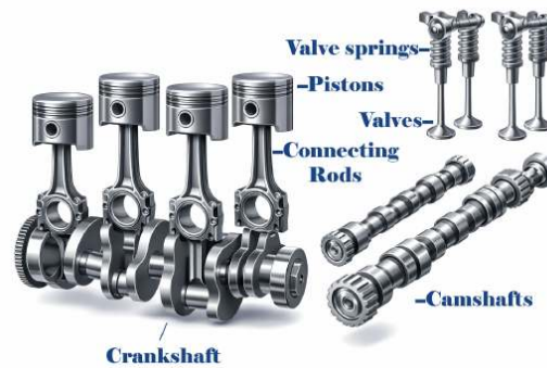
Figure 2.3.2 Pistons, connecting rods, crankshaft, camshaft, valves
