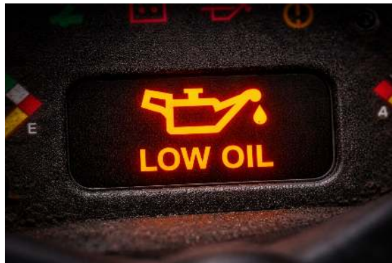
Figure 8.6.1 Dashboard warning light indicating "LOW OIL" with an oil can icon and a droplet, glowing in bright orange.
