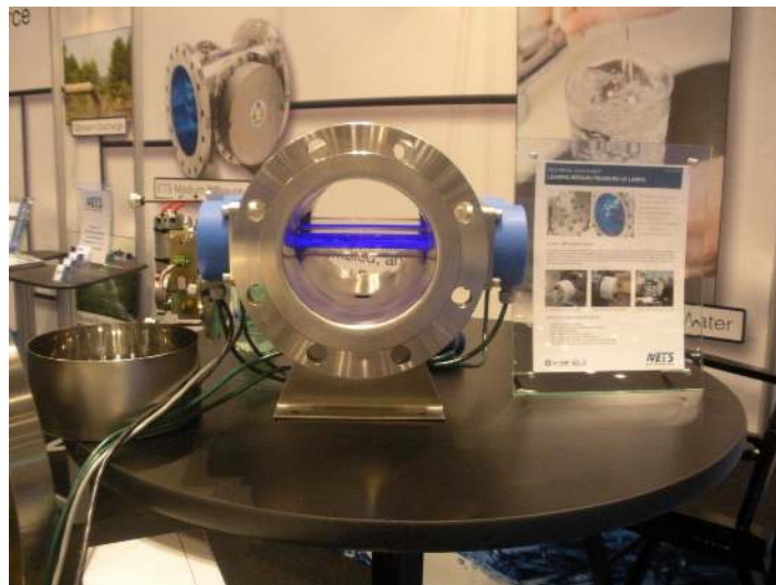
Figure 3.1: UV light used for disinfection in water treatment.
