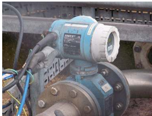
Figure 1.5.4: Magnetic Flow Meter by Mtaylor848 is licensed under CC BY-SA 3.0
