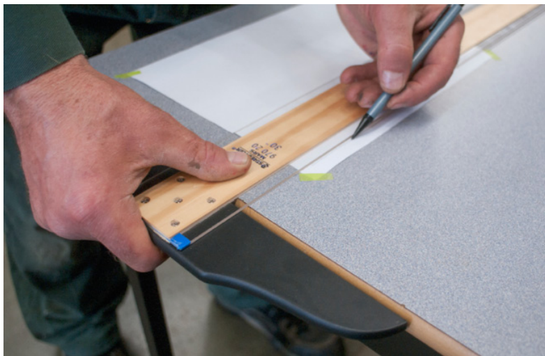
Figure 1.3.1.1: A person using a T-square
