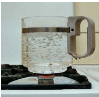
Figure 1.2.5: Boiling Water. When liquid water boils to make gaseous water, it undergoes a phase change. (CC BY-SA 3.0 Unported; Markus Schweiss via Wikipedia)
