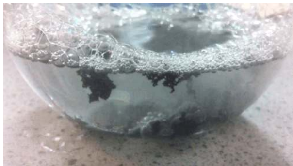
Figure 5.4.1: Zinc Metal plus Hydrochloric Acid. It is fairly obvious that zinc metal reacts with aqueous hydrochloric acid! The bubbles are hydrogen gas (right side of Equation 5.4.1).
